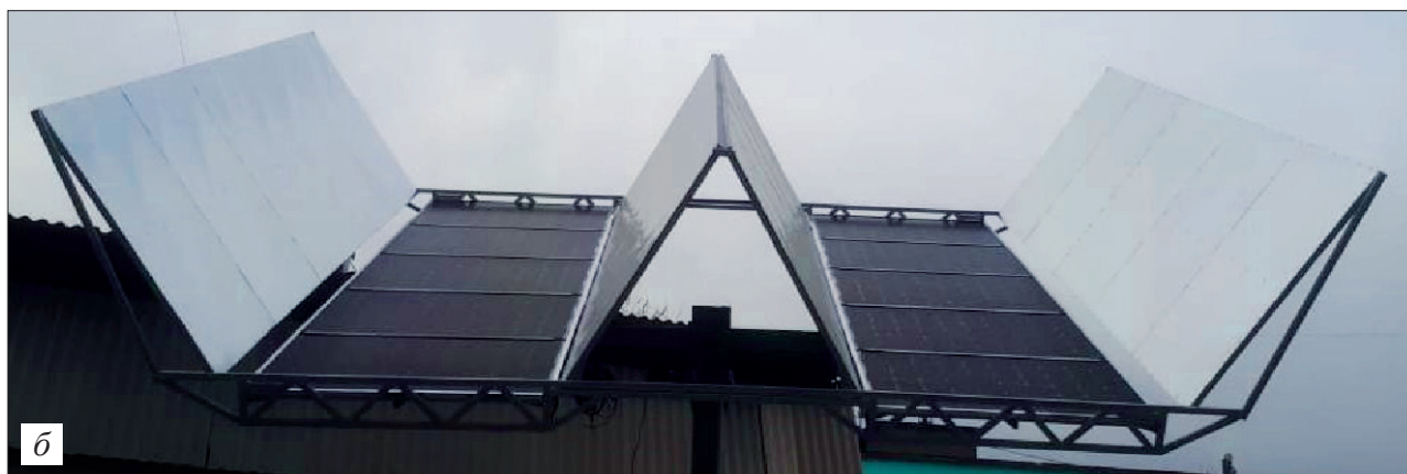
Fig. 1. Configuration of light-collecting system for mobile photovoltaic converter on the basis of advanced solar cells: (a) general appearance, (b) photoelectric converter in expanded condition, (b, r) system assembly steps
